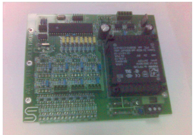
Figure 9. The digital recording module using the microcontroller with integrated port analog-digital converter.
